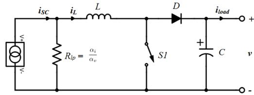
Fig. 4: linearized PV connected to boost converter
