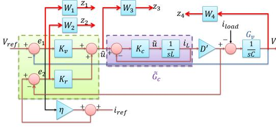
Fig. 3: Block diagram representation of the inner-outer control design. The regulated variables  $z_1, z_2, z_3$  and  $z_4$  correspond to weighted - (a) tracking error in DC-link voltage, (b) mismatch between  $i_{ref}$  and  $i_{load}$ , (c) control effort  $\hat{u}$ , and (d) output voltage tracking, respectively.
