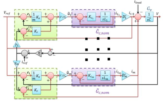
Fig. 4: Many-converters system with shaped inner plants  $\tilde{G}_c$ . In the proposed implementation, we adopt the same outer controller for different converters, i.e.,  $K_{v_1} = K_{v_2} = \dots = K_{v_m} = \frac{1}{m} K_v$  and  $K_{r_1} = K_{r_2} = \dots = K_{r_m} = K_r$ ;  $\gamma_k$  represents the proportion of power demanded from the  $k^{\text{th}}$  source.
